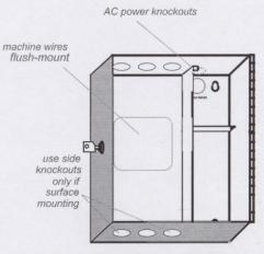
FIGURE 3: Mounting & Knockouts
