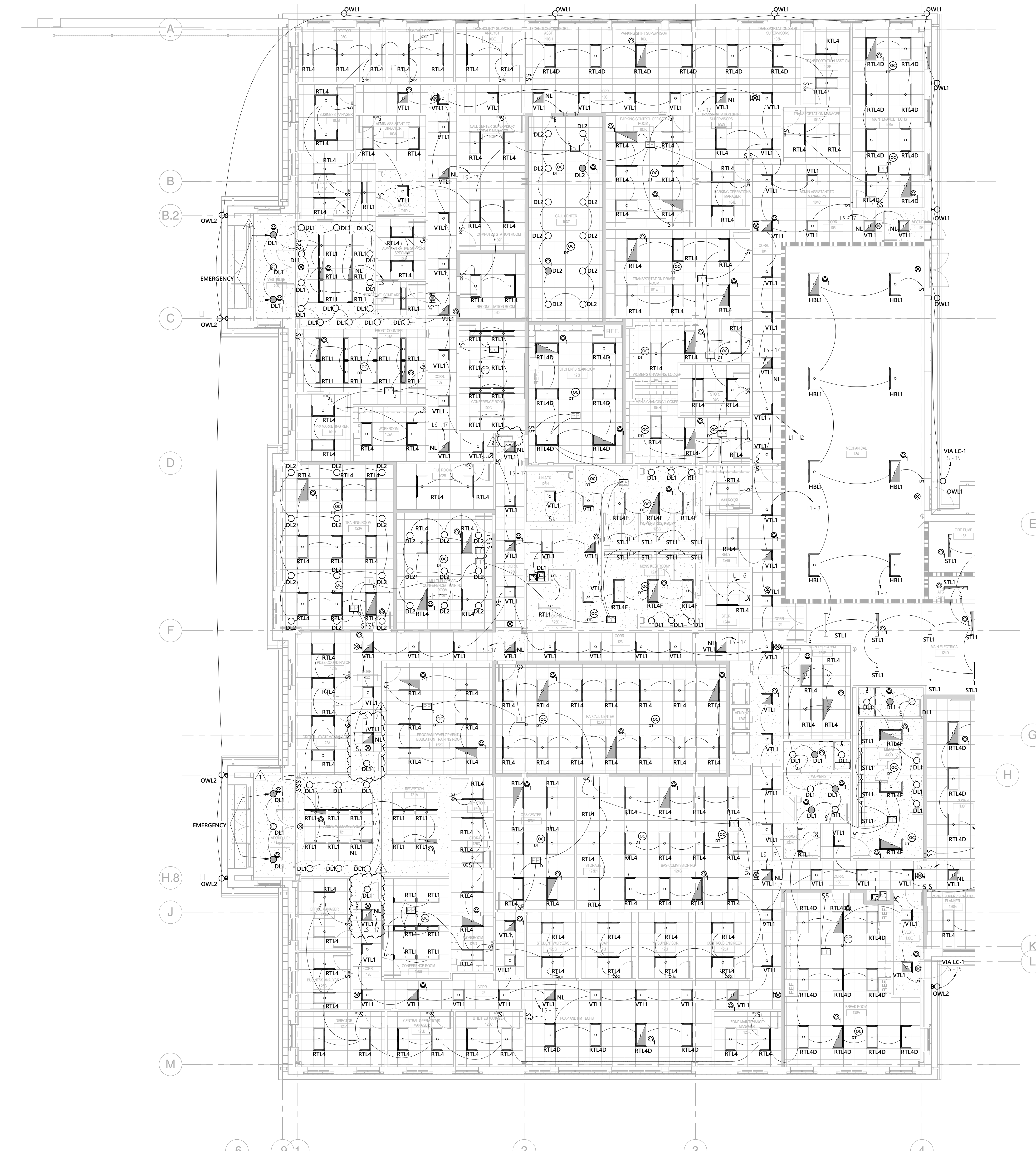
1 OFFICE/SHOPS - REFLECTED CEILING PLAN - PATS/FO - LIGHTING 1/8" = 1'-0" SCALE: 1/8"=1'-0"
